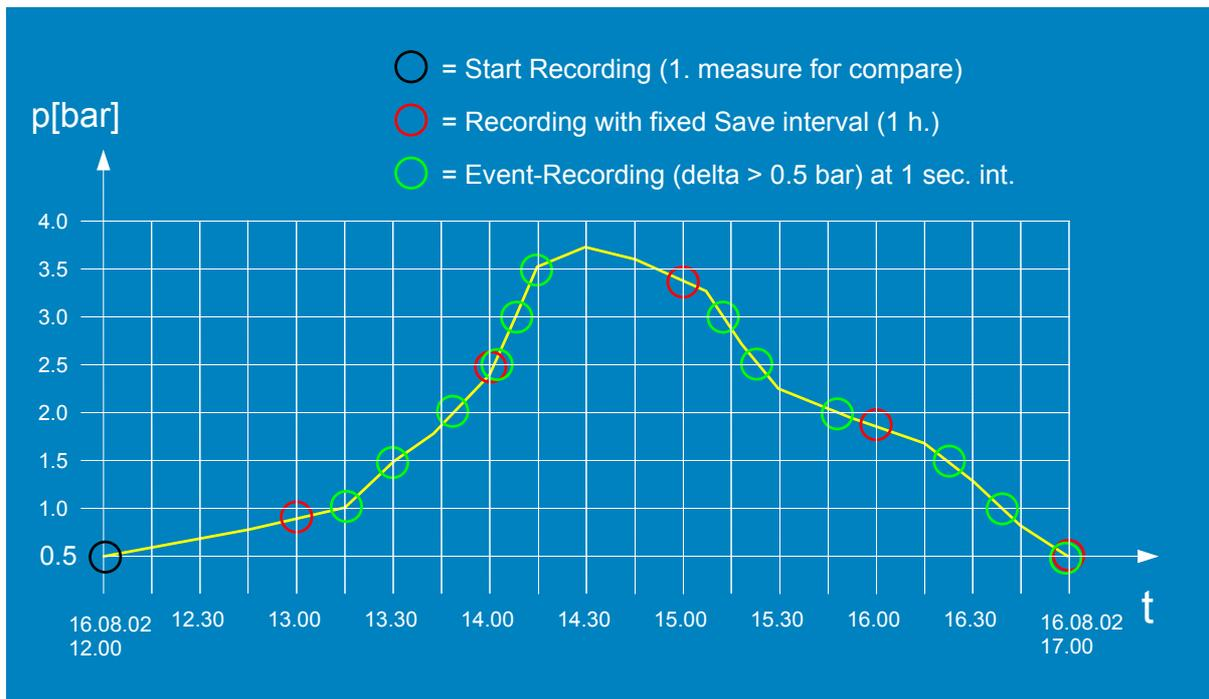
As soon as the configuration has been written into the device, a first measured value is recorded (in the sample: Start recording at 12.00 p.m.). As per configuration, this measured value is compared every second with the current measured value, till the difference is 0.5 bar. This first happens at 13.15. The next recording takes place at 13.30, etc... Independent of that, each fixed Save-Interval (1 hour), an additional recording is done.
