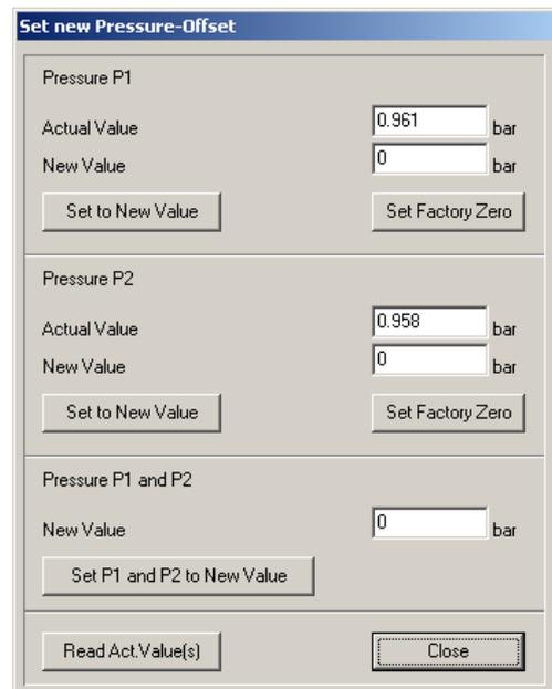
To reset a sensor to its factory setting, click **Set Factory Zero** respectively.
