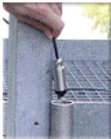
The level sensor, connected by a cable to the electronics housing, is immersed into the pipe. The housing incorporates the electronics, the battery and the air pressure sensor.
