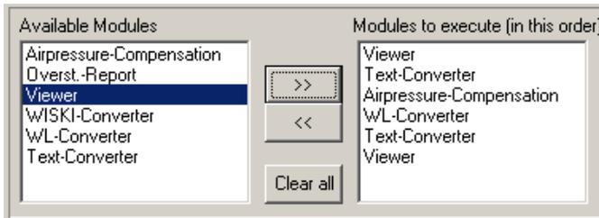
After selecting the recordings to be read out and modules to be executed, the read-out procedure is initiated by clicking **Read Record(s)**.
