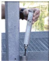
The electronics housing is mounted onto the end of the pipe. The protective cap of the interface must be cleaned from dirt and water prior to removing.
