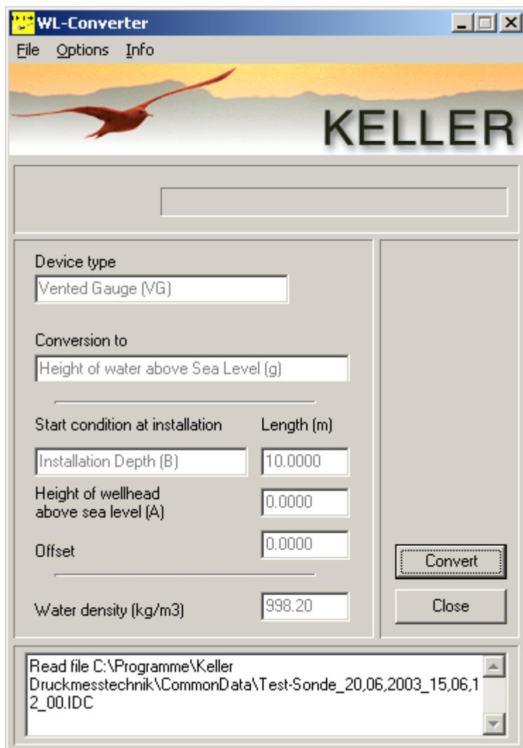
Clicking **Convert** leads to all measured values being converted into water levels. The unit for converted values is always meter (m).
