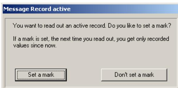
If a mark is set, a new recording starts. This means that at the next read-out of the active recording (only No. 1) only data recorded after the mark was set is included in the read-out.
